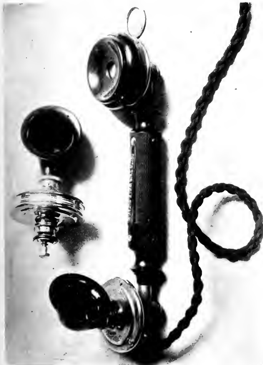
FIG. 35.—ERICSSON COMBINED TRANSMITTER AND RECEIVER.
